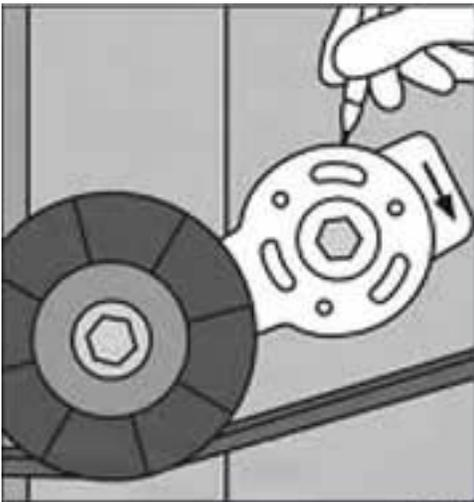
FIGURE 11: TENSIONER MARKING
